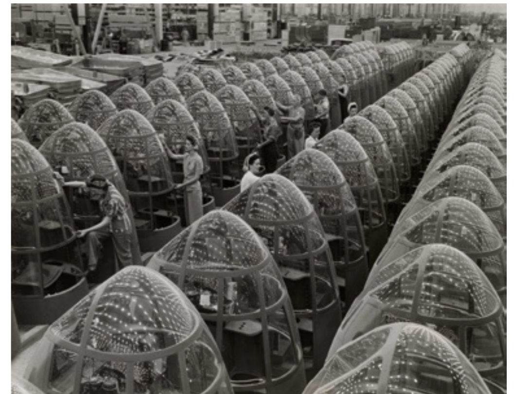
Below: Women aircraft workers finishing transparent bomber noses for fighter and reconnaissance planes at Douglas Aircraft Company’s plant in Long Beach, California, 1942. Picture by Alfred Palmer
